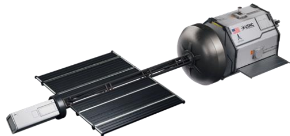
Figure 3: DIU concept spacecraft utilizing 1kW e EmberPower for power system and electric propulsion.
