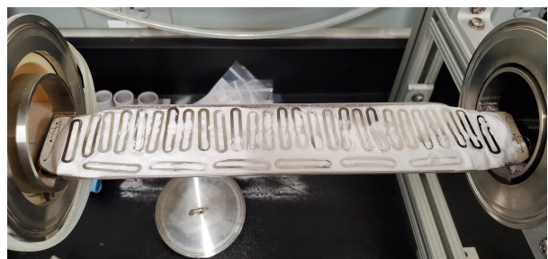
Figure 8: Bulk heat-treatment of ferromagnetic foils for fluxgate cores.
