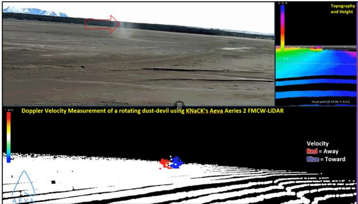
Figure 2: Example data collected by the FMCW-LiDAR sensor on KNaCK (Aeva Aeries 1). This is a still-image snippet of real-time video of rotating dust-devil a glacial sand playa near the Holuhraun flow during the NASA PSTAR Rover and Aerial Vehicle Exploration Network (RAVEN) field campaign in July 2022. The HD Video image (upper left) shows a dust-devil moving from right to left (~S to N). Topography and height (upper right) shows the general topography and slope of the surface and the height of the positive relief of the dust-devil. The velocity-data (bottom) shows the Doppler velocity of the rotating vortex of the dust-devil rotating clockwise. Blue regions are moving toward, red regions are moving away from the sensor (white is no relative motion). Note that the sensor can measure the speed and direction of the vortex. These proof-of-concept results indicate that small-scale atmospheric phenomena can be studied in unprecedented detail, while also providing rover position and navigation data, and topography and morphology mapping data.
