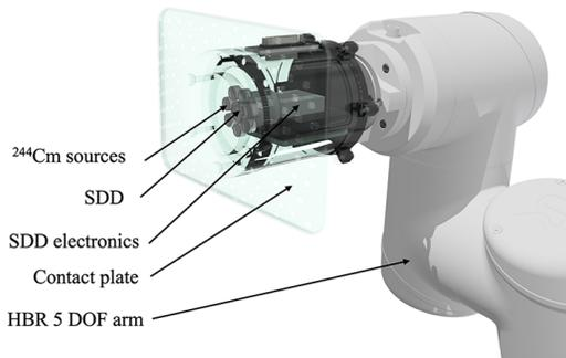
Fig. 1: LunaPIX Arm Unit attached to the HoneyBee Robotics robotic arm. During an analyses, a contact plate (translucent in this image) is pressed onto the regolith. An SDD and six <sup>244</sup>Cm sources can be seen recessed from the contact plate.
