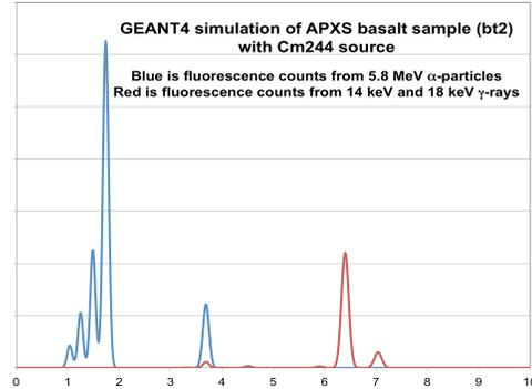
Fig. 2: Simulated spectrum of APXS basalt sample bt2, calculated using GEANT4 and a Fundamental Parameters model of LunaPIX. Red spectrum =  $\gamma$ -ray fluorescence, blue spectrum =  $\alpha$ -particle fluorescence (30 mCi <sup>244</sup>Cm).
